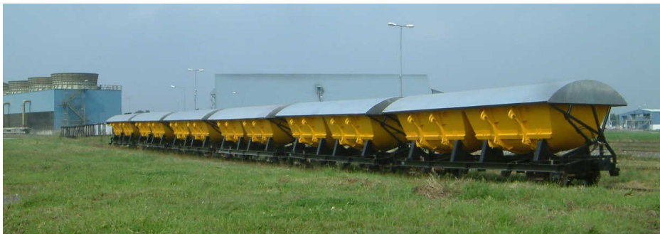
Plate 1: Ash wagon of a rail bogey with two ash buckets and a hydraulically controlled lid
